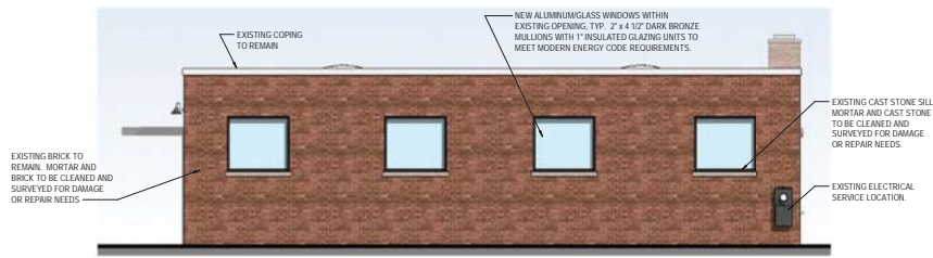
2 BUILDING EXTERIOR ELEVATION - SOUTH SCALE: 1/8" = 1'-0"
