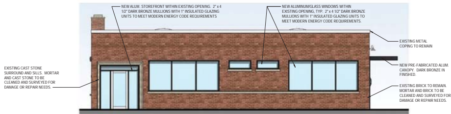
1 BUILDING EXTERIOR ELEVATION - NORTH SCALE: 1/8" = 1'-0"
